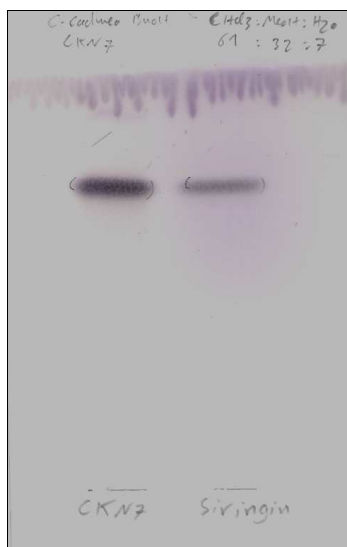
Picture 1. TLC profile of compound 3 (syringin) (silica gel plate, \text{CHCl}_3/\text{MeOH}/\text{H}_2\text{O} , 61:32:7)
