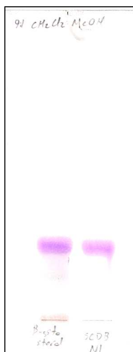
Picture 2. TIC profile of compound 5 ( \beta -sitosterol-3- O - \beta -D-glucopyranoside) (silica gel plate, \text{CH}_2\text{Cl}_2/\text{MeOH} , 9:1).
