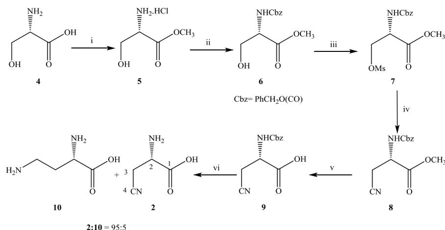
**Scheme 2.**  $\beta$ -Cyano-L-alanine *via* L-serine. (i) AcCl, MeOH, 0°C  $\rightarrow$  reflux, 2 h, 100%; (ii) PhCH<sub>2</sub>O(CO)Cl, NaHCO<sub>3</sub>, THF, 0°C  $\rightarrow$  rt, 3 h, 66%; (iii) CH<sub>3</sub>SO<sub>2</sub>Cl, NEt<sub>3</sub>, dry CH<sub>2</sub>Cl<sub>2</sub>, 0°C  $\rightarrow$  rt, 3 h, 92%; (iv) NaCN (or K<sup>13</sup>CN), dry DMF, rt, 14 h, 76%; (v) KOH, EtOH, rt, 3 h, then 4 M HCl 72%; (vi) H<sub>2</sub>/Pd-C, MeOH, rt, 14 h, 37%.
