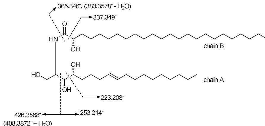
**Figure 2.** Selective fragmentation patterns in the mass spectra of compound **1** (trolliamide) isolated from *E. tonkinensis*. MS spectra were recorded using a Shimadzu LCMS-IT-TOF instrument at atmospheric pressure chemical ionization (APCI) conditions.
