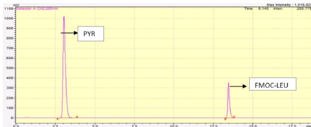
Figure 3. Chromatogram of mixture in MPA: 0.1% OPA in Water MPB: ACN at 285nm in Zodiac;4.6 ID *250mm; C18; 5 \mu m
