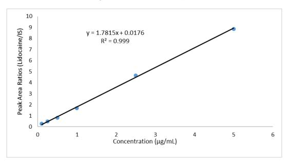
Figure 3. Calibration curve of the GC-FID method
