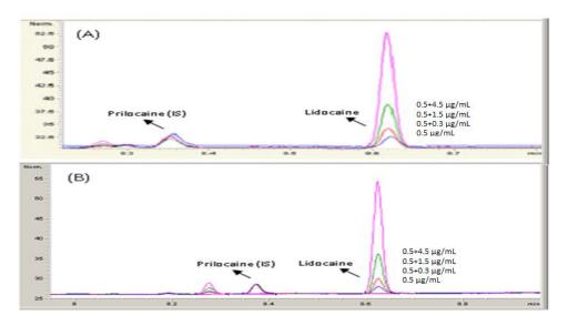
Figure 5. GC-FID chromatograms of Jetokain (A) and Jetmonal (B) injection samples
