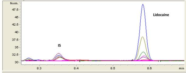
Figure 2. GC-FID Chromatograms of standard solutions of lidocaine and IS.
