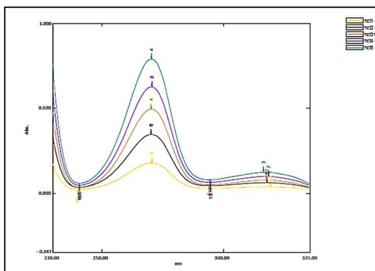
**Figure 3.** Overlain spectra of HCT (2.5-12.5  $\mu\text{g/mL}$ )
