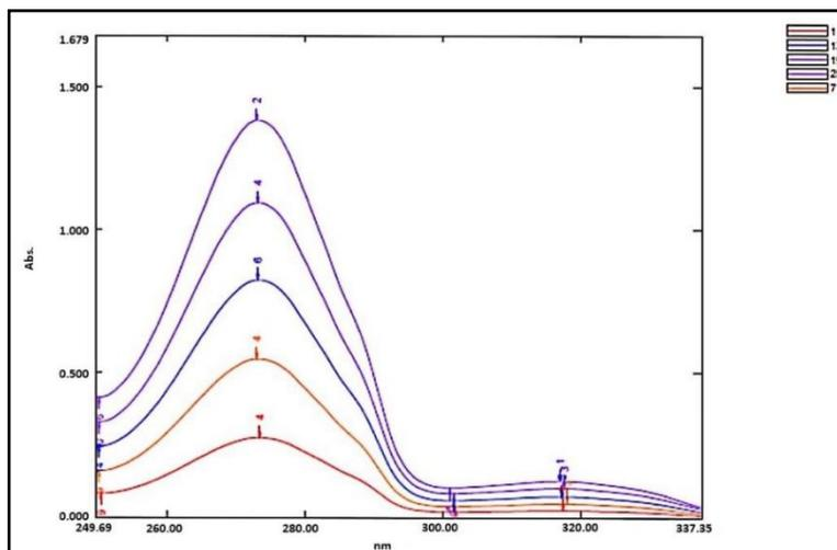
**Figure 4.** Overlain spectra of ALI (30, 60, 90, 120 and 150 µg/mL) and HCT (2.5, 5, 7.5, 10 and 12.5 µg/mL) sample
